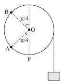
Between P to A the pulley accelerates as torque due to tension will exceed the torque due to  $m_0g$ . Between A to B the pulley system retards and beyond B it will once again accelerate.
